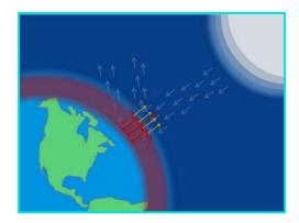
This is a screenshot of the second greenhouse gas effect slide. It features a representation of the earth emitting longwave radiation arrows, and greenhouse gases re-emitting the radiation with red arrows and warming the atmosphere and surface.
